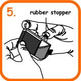
After refilling is completed, clean the ink inlet hole with tissue paper and seal it with rubber stopper provided. Ensure ink is not dripping from nozzle. Ink will drip if rubber stopper is not inserted or seated firmly onto the hole.
