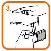
Place tip of plunger on "plastic ball" or "rubber stud" and hammer plunger to push the "plastic ball" or "rubber stud" into cartridge.
