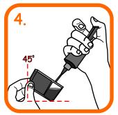
Hold the cartridge at 45° angle in the direction as shown in picture. Insert needle slowly into cartridge and press the plunger to inject ink as follow: **PGI 5B = 11-13ml of ink**
