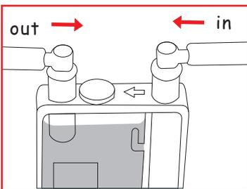
4. Attach the end of PIPELINE No. (1) to the 'IN' ELBOW TUBE properly for each color.
