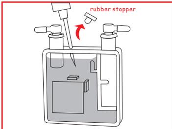
2. Pull out the RUBBER STOPPER on the DAMPER. Push the needle into the DAMPER and slowly fill up the DAMPER with ink until its 95% full. Then, re-insert the RUBBER STOPPER. Follow this step in filling up each ink color (BCMY) into each DAMPER.
