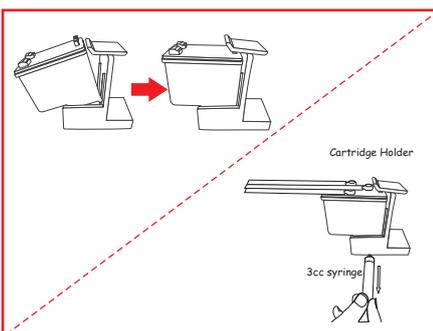
7. Insert the cartridge into the HOLDER and push the top of the cartridge all the way until you hear it "clicking". Connect the 3cc syringe to the rubber holder of the HOLDER and slowly suck out 0.5ml of ink from the cartridge. Remove the cartridge from the holder and clean the excessive ink around the nozzle, dabbing the nozzle pat on soft tissue. Then, install the cartridge into the printer. Properly fix up the CISS tank to the printer.
