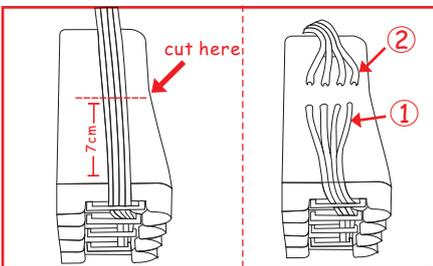
3. Use a scissor to cut the PIPELINE about 7cm from the end of one side of CISS tank. The PIPELINE will become into 2 parts.
