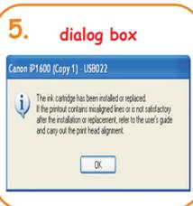
Install the cartridge back into the printer. Do a nozzle check. Click OK when this dialog box is shown. If the result of the nozzle check is not good, execute deep cleaning and check print out. Repeat deep cleaning if necessary.
