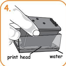
4. Dip the print head of the cartridge into water for 10 seconds.
