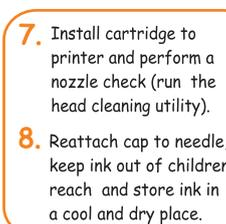
7. Install cartridge to printer and perform a nozzle check (run the head cleaning utility).
