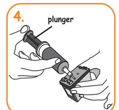
4. Push the needle straight into the cartridge and pull out a little (2mm). Slowly press the plunger to inject about 3ml per color of ink into the cartridge. Ensure cartridge is in upright position.
