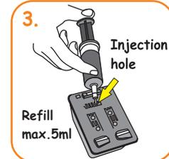
3. Push the needle straight into the cartridge and pull out a little (2mm). Slowly press the plunger to inject about 5ml of ink into the cartridge. Ensure cartridge is in upright position. Stop filling if ink start to drip at print head.
