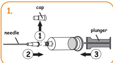
1. Remove the cap then attach the needle to the ink tube. Fix the plunger (per diagram) to allow ease of pressing.
