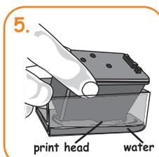
5. Dip the print head of the cartridge into water for 10 seconds.
