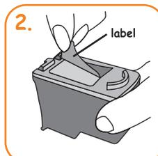
2. Remove the label on the cartridge.
