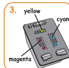
3. Study the position of the color and ensure the right color ink is injected into cartridge.
