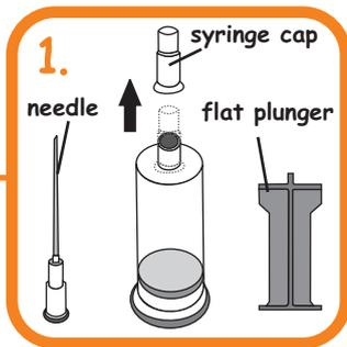
Setup the "Injection Tube" by removing the syringe cap then attach the needle & plunger to the ink tube.
