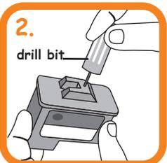
Drill a hole on the color cap of the cartridge.
