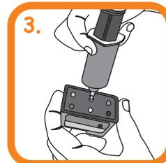
Push the needle into the cartridge and pull out a little (2mm). Slowly press the plunger to inject 8-10ml of ink into the cartridge. Ensure cartridge is in upright position. Stop filling if ink start to drip at print head.
