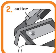
Slit the color lid and base at the 4 corners of the cartridge using a cutter.
