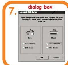
Install cartridge to printer. Run the printer utilities and at dialog box, select "new cartridge".
