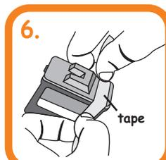
Reattach the lid to the base and hold it on with the tape provided.
