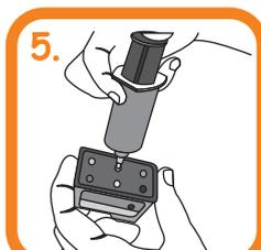
Push the needle into the cartridge and pull a little (2mm). Slowly press the plunger to inject 3-5ml of ink into the cartridge. Ensure cartridge is in upright position. Stop filling if ink start to drip at print head.
