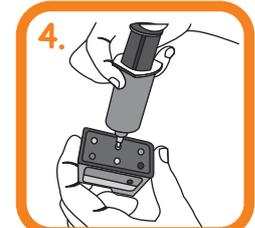
Push the needle into the cartridge and pull out a little (2mm). Slowly press the plunger to inject 3-5ml of ink into the cartridge. Ensure cartridge is in upright position. Stop filling if ink start to drip at print head.
