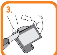
Pry open the color lid with cutter to remove it from the base.
