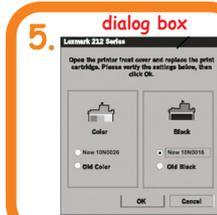
Install cartridge to printer. Run the printer utilities and at dialog box, select "new cartridge".
