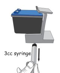
Connect the syringe 3cc to the rubber hole of the holder and slowly suck out about 0.5ml of ink from the cartridge. Remove the cartridge from holder and clean the excessive ink around the nozzle, dabbing the nozzle part on soft tissue. Install the cartridge into the printer, and run "head cleaning" process before use.
