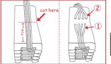
3.Use a scissor to cut the PIPELINE about 7cm from the end of one side of CISS tank. The PIPELINE will become into 2 parts.
