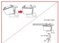
7. Insert the cartridge into the HOLDER and push the top of the cartridge all the way until you hear it "clicking". Connect the 3cc syinge to the rubber holder of the HOLDER and slowly suck out 0.5ml of ink from the cartridge. Remove the cartridge from the holder and clean the excessive ink around the nozzle, dabbing the nozzle pat on soft tissue. Then, install the cartridge into the printer. Properly fix up the CISS tank to the printer.
