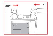
4. Attach the end of PIPELINE No. (1) to the 'IN' ELBOW TUBE properly for each color.
