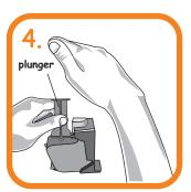
Place tip of plunger on metal ball and hammer plunger to push ball into cartridge.
