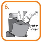
Seal hole with rubber stopper provided.
