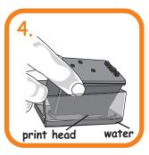
Dip the print head of the cartridge into water for 10 seconds.
