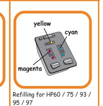
Study the position of the color and ensure the right color ink is injected into cartridge.
