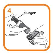
Push the needle straight into the cartridge and pull out a little (2mm). Slowly press the plunger to inject about 3ml per color of ink into the cartridge. Ensure cartridge is in upright position.
