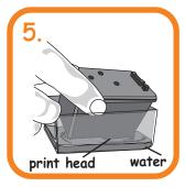
Dip the print head of the cartridge into water for 10 seconds.
