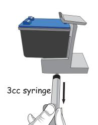
Connect the syringe 3cc to the rubber hole of the holder and slowly suck out about 0.5ml of ink from the cartridge. Remove the cartridge from holder and clean the excessive ink around the nozzle, dabbing the nozzle part on soft tissue. Install the cartridge into the printer, and run "head cleaning" process before use.
