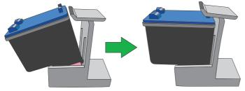
Insert the cartridge into the holder and push the top of the cartridge all the way in until you hear it clicking.
