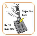
Push the needle straight into the cartridge and pull out a little (2mm). Slowly press the plunger to inject about 5ml of ink into the cartridge. Ensure cartridge is in upright position. Stop filling if ink start to drip at print head.
