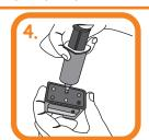
Push the needle into the cartridge and pull out a little (2mm). Slowly press the plunger to inject 3-5ml of ink into the cartridge. Ensure cartridge is in upright position. Stop filling if ink start to drip at
