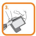
Ply open the color lid with cutter to remove it from the base
